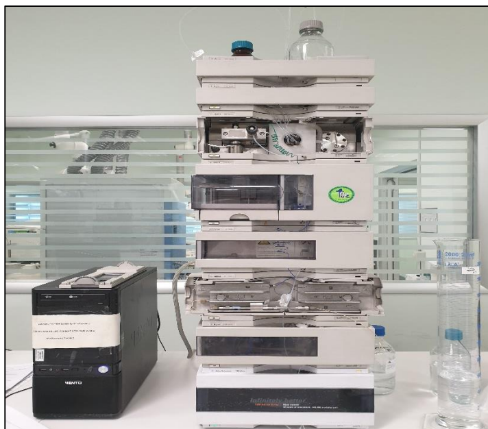
Figure 2.2. Agilent Series 1100 High- Performance Liquid Chromatography – HPLC
