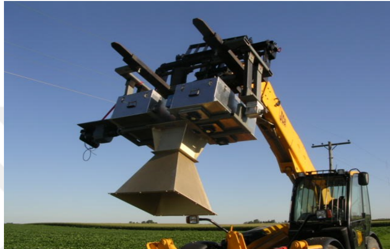
Figure 8. ISU radiometer on a lifter. Receiver and power supplies are contained in two separate boxes mounted on the sides of antenna orthomode
