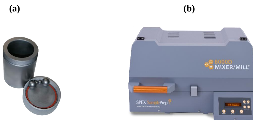
Figure 3.1 (a) Milling vial with stainless steel balls and (b) high energy ball milling device.
