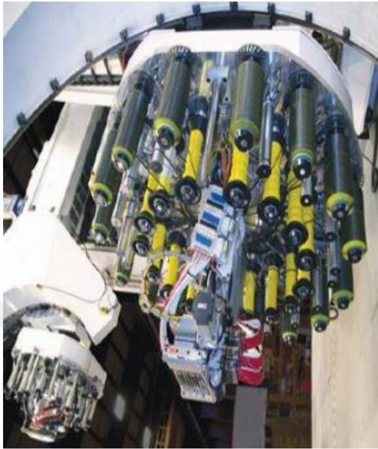
Figure 2.12 AFP machine head with multiple towes
