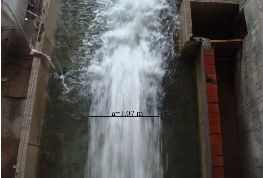
Figure 30 Width of the dispersed jet for Q = 0.13 \text{ m}^3/\text{s}
