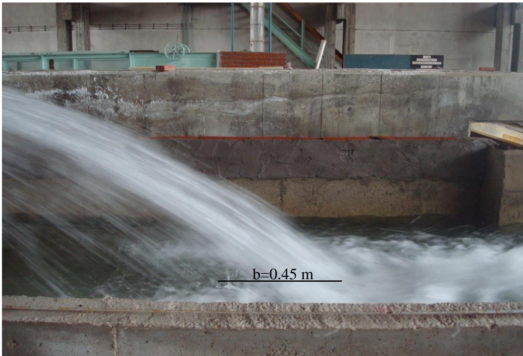
Figure 35 Length of the dispersed jet for Q = 0.07 \text{ m}^3/\text{s}
