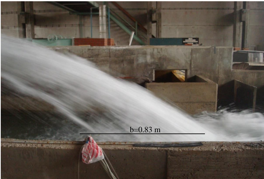
Figure 27 Length of the dispersed jet for Q = 0.19 \text{ m}^3/\text{s}
