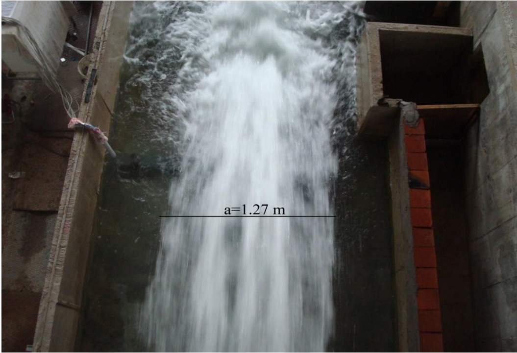
Figure 26 Width of the dispersed jet for Q = 0.19 \text{ m}^3/\text{s}
