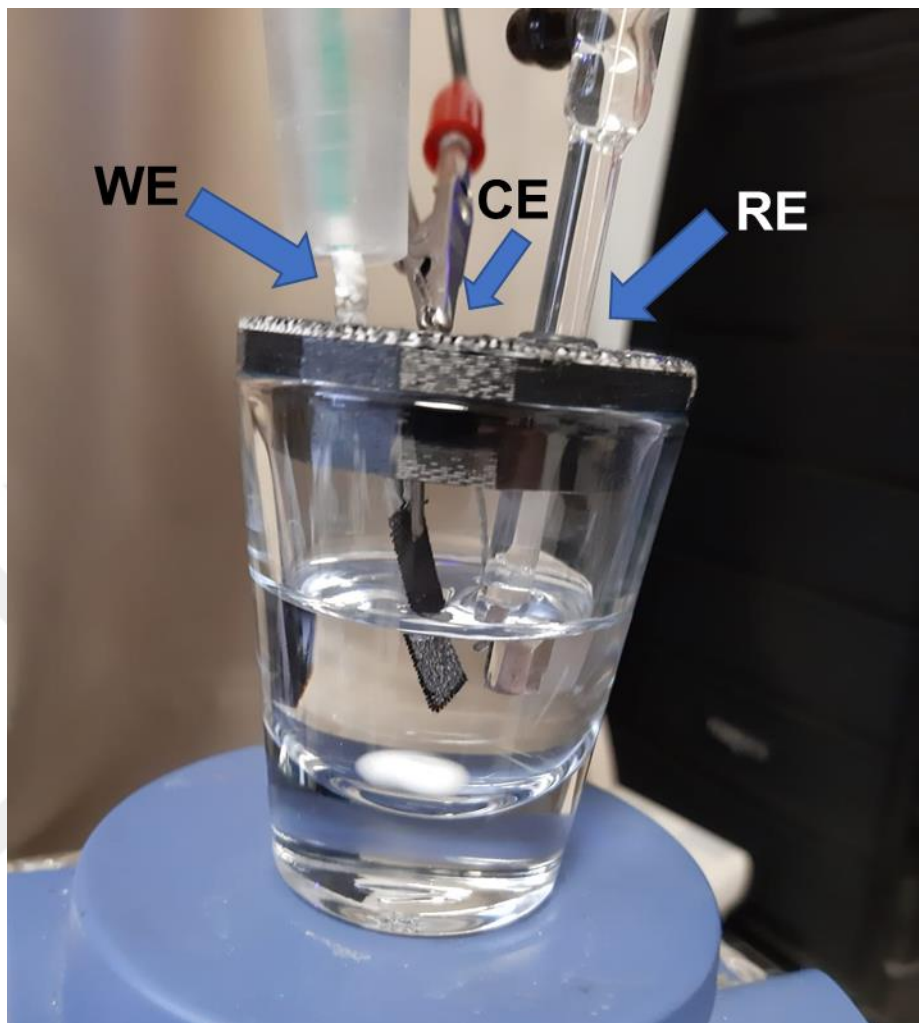
Figure 2.1 The three-electrode configuration electrochemical setup. WE, RE and CE denote working electrode, reference electrode and counter electrode, respectively.
