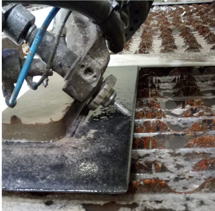
Figure 4.1. The Picture While the Composite Plate Cutting with Robotic Water-Jet Machine
