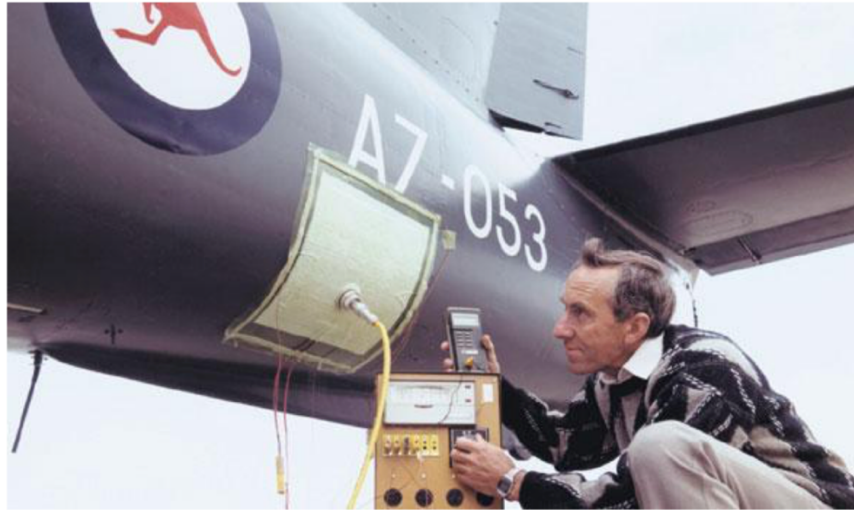
Figure 1.1. Repair of an airframe with a patch [6]
