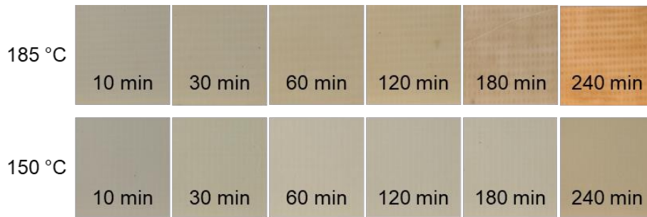
Figure 4.12: Color change in PCB substrates after PMC operations with different temperatures and times
