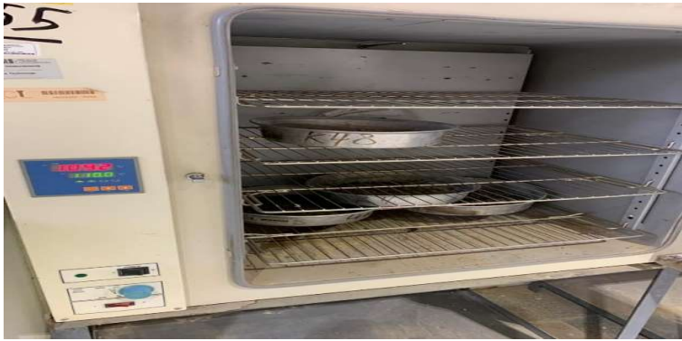
Figure 3.6. Thermostatically controlled oven dry for OMC
