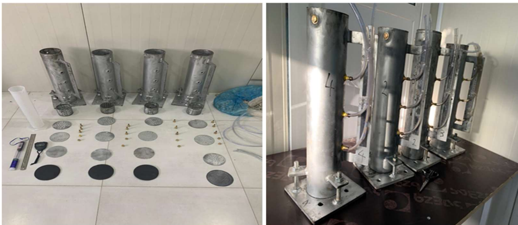
Figure 3.10. The applied permeability test device
