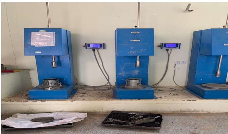
Figure 3.7. Compaction testing machine
