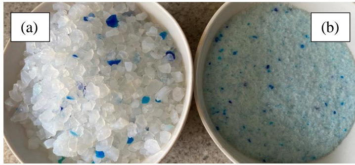
Figure 6.6 Photo of original silica sand (a) and ground silica sand (b)
