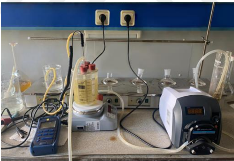
Figure 6.1 Fully mixed crystallizer setup used in experimental studies (Personal archive, 2022)
