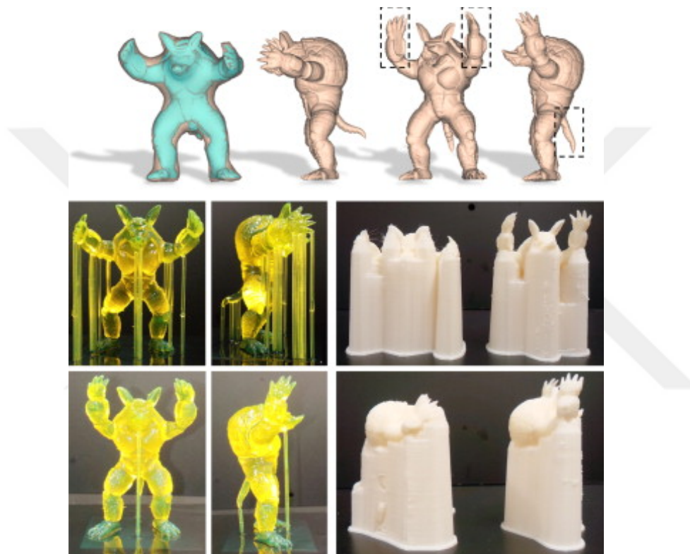
Figure 2.6: Support volume reduction by modification [15]
