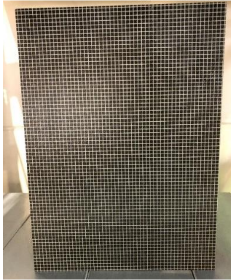
Figure 3.10 Produced composite plate 450 x 650 x 2.61 mm in size
