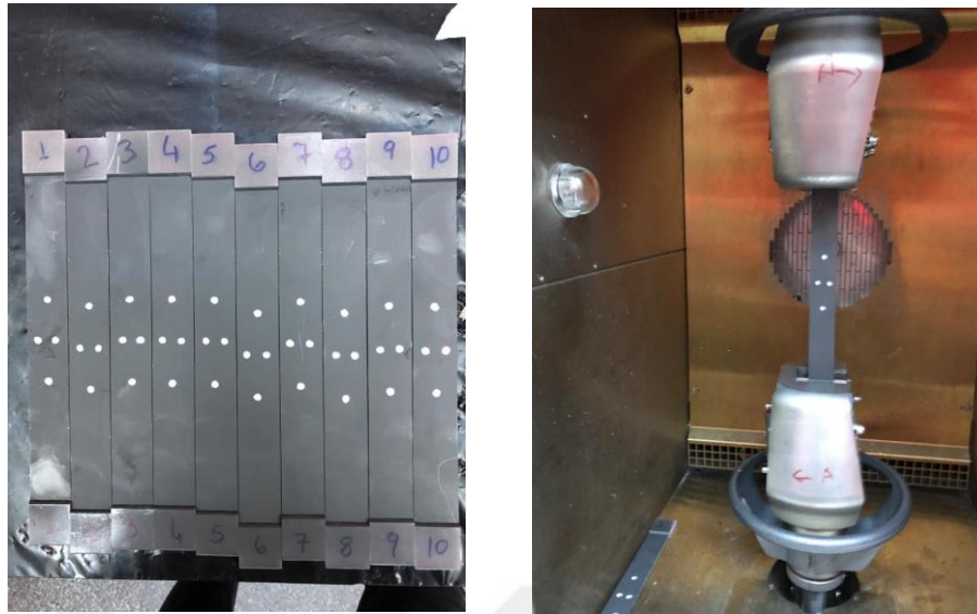
Figure 3.8 Shear test coupons which were marked to measure both longitudinal and lateral strain
