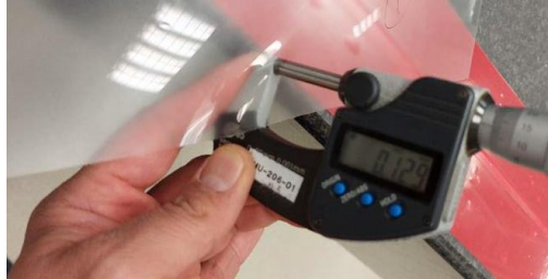
Figure 3.3 PES film thickness measurement with micrometer
