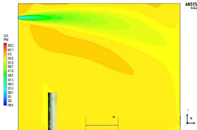
Figure 5.32: CO 2 Concentration contour, 2.0 m/s in the section (A).
