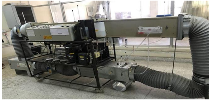
Figure C.8: Air conditioning laboratory unit, A660/15611.
