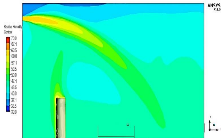
Figure 5.29: Relative Humidity contour, 1.0 m/s in the section (A)
