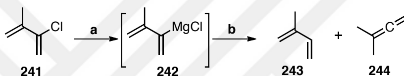
Scheme 2.27: The formation of Grignard 242 reagent and its protonolysis products. Reagents and conditions: (a) Magnesium powder (2.9 mol equiv), \text{BrC}_2\text{H}_4\text{Br} (0.70 mol equiv), \text{ZnBr}_2 (0.030 mol equiv), THF, reflux, 75 min, 55%. (b) Quenched with water and diluted with \text{CDCl}_3 , (ratio 243 : 244 , 90:10).
