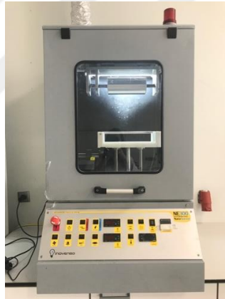
Figure 3. 5: NanoSpinner NE300 model electrospinning device.
