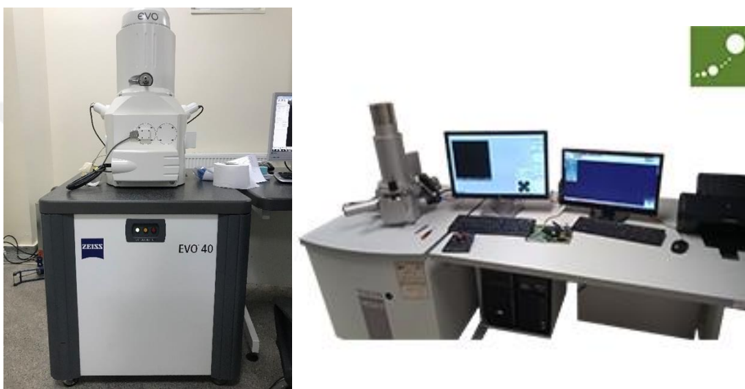
Figure 3. 7: SEM devices used for nanofiber image analysis ZEISS EVO 40 a), TESCAN - VEGA4 - W source and EDX b), respectively.
