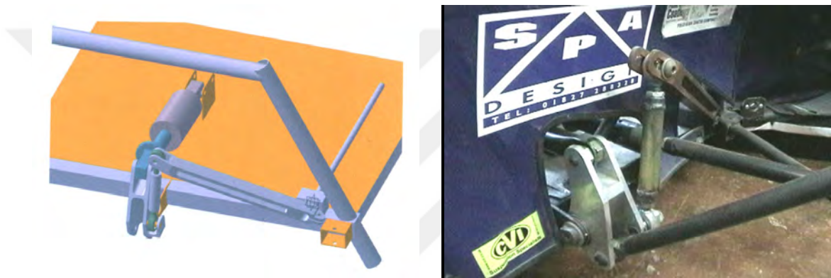
Figure 6.7 CAD design of the front suspension's damper and anti roll bar placement
