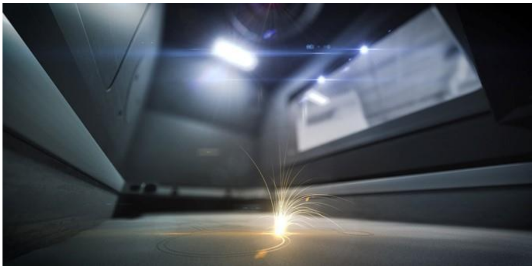
Figure 2.6 : Laser melting phase of LPBF process [71].
