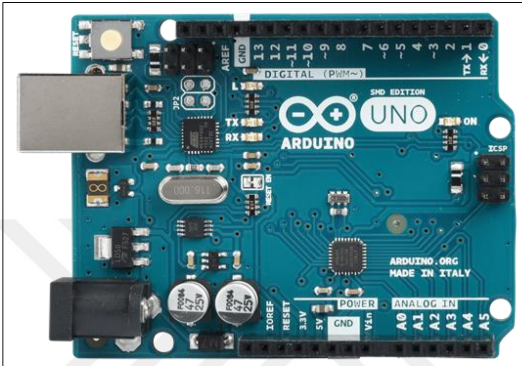
Figure 2.2: Arduino Uno Development Board [9]
