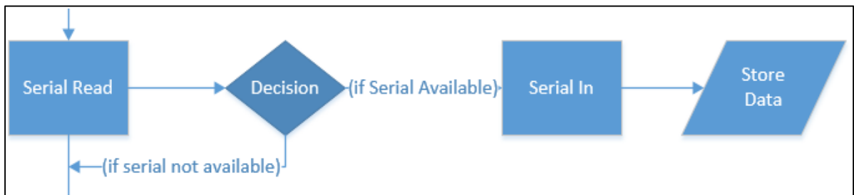
Figure 2.11: Serial Read Flowchart [17]
