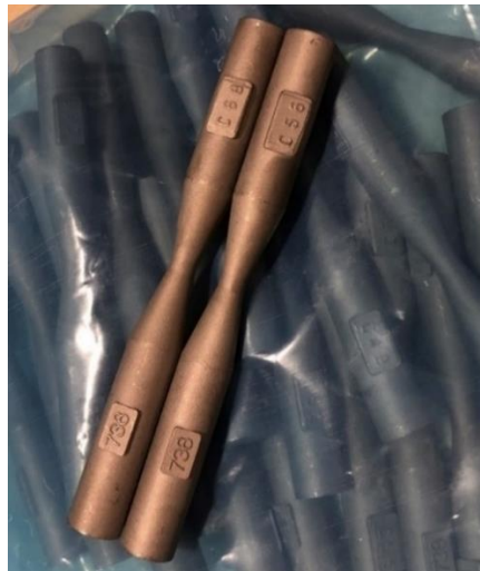
Figure 2.2: Blank sample produced by vacuum investment casting
