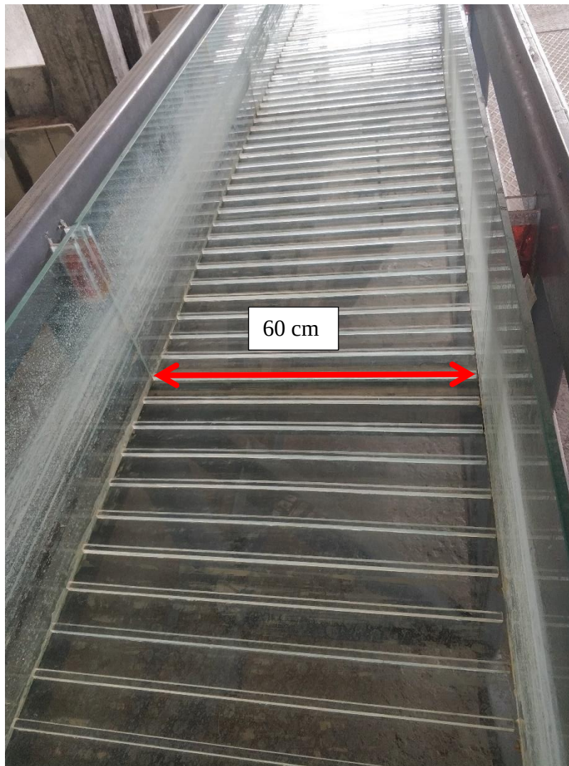
Figure 3.3 Square Bars Placed on the Channel Bed
