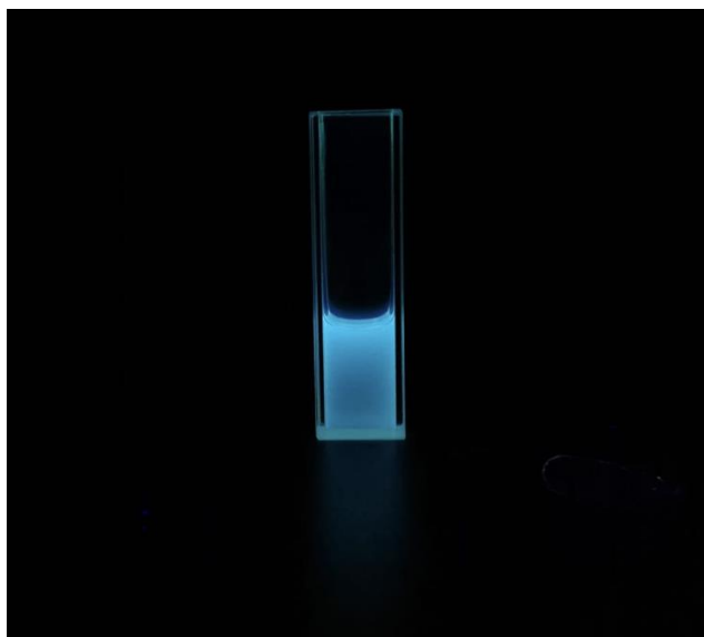
Figure 3.2 : 24 h CdSSe ternary alloyed quantum dots under UV lamp with 366 nm UV-irradiation.
