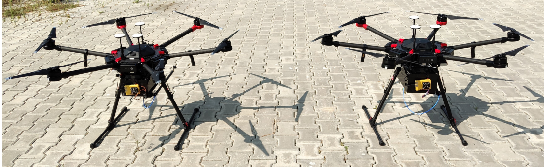
Figure 5.2 : Illustration of the measurement campaign in which two commercially available hexacopter are used as transmitter and receiver. Note that two drones are ready to take-off with mounted channel measurement box.
