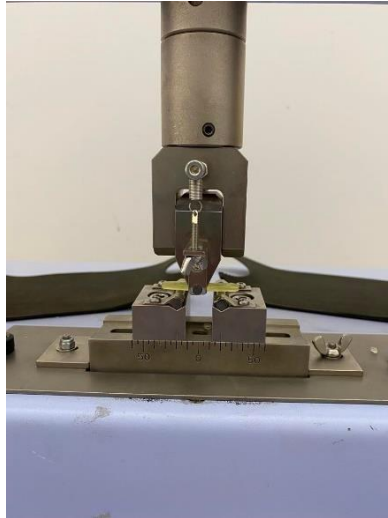
Figure 3.18: SHIMADZU AG-IC used to perform three-point bending test of dental filling composites
