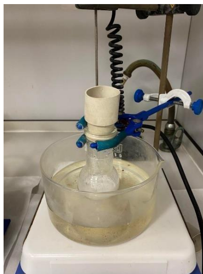
Figure 3.6: The reaction of synthesis of Si/PMMA core/shell structure
