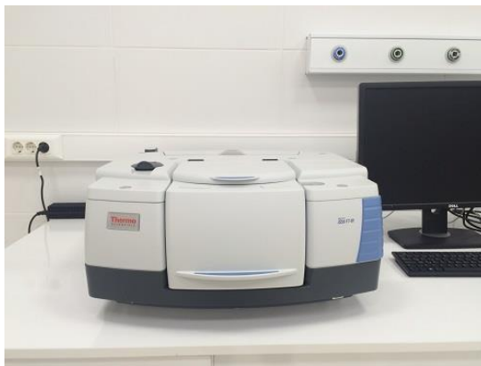
Figure 3.12: Thermo Scientific Nicolet iS50 FT-IR used for FT-IR analysis of synthesized NPs
