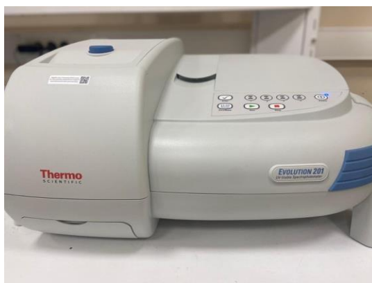
Figure 3.14: Thermo Scientific Evolution 201 UV-Visible Spectrophotometer used to measure the absorbance of the synthesized NPs
