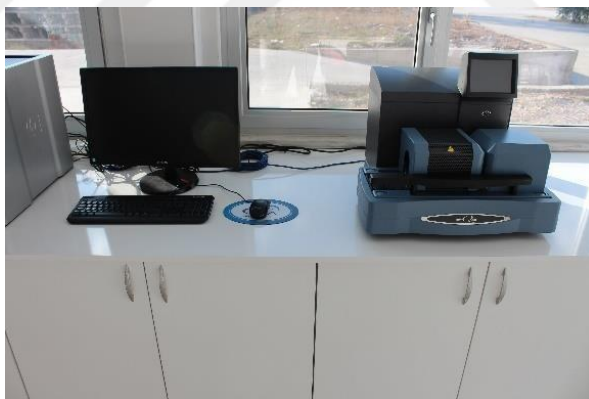
Figure 3.15: TA TGA-SDT Q600 used to measure the thermal stability of the synthesized NPs
