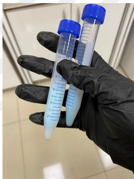
Figure 3.4: Synthesized Si-NPs after purification, inside C_2H_5OH
