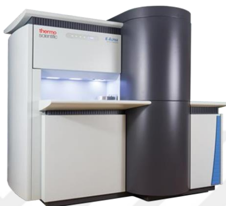
Figure 3.16: Thermo Scientific K-Alpha XPS device used to determine the elemental composition of the synthesized NPs
