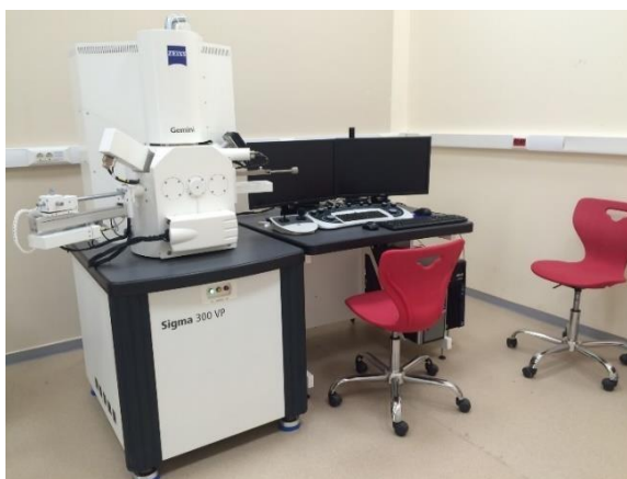
Figure 3.13: Carl Zeiss 300VP used for SEM characterization of synthesized NPs
