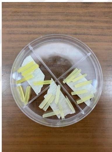
Figure 3.19: The dental filling composite parts obtained after the three-point bending test
