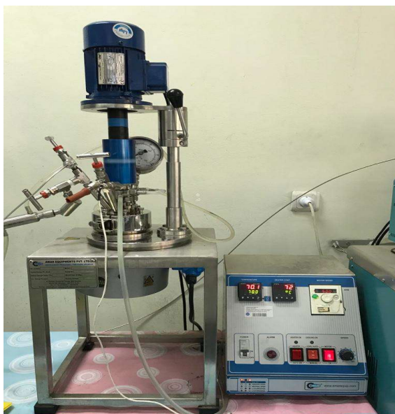
Figure 4.6: Catalytic wet air oxidation experimental set-up
