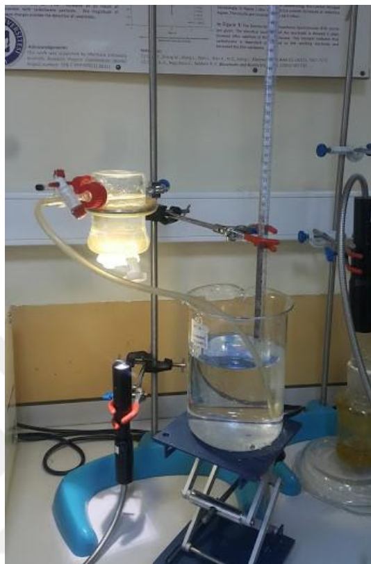
Figure 3.11 Photocatalytic hydrogen production system
