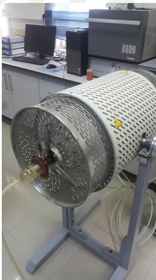
Figure 2.1 Protherm tube furnace
