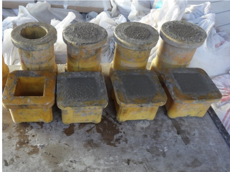
Figure 3.7 Filling the molds with fresh concrete
