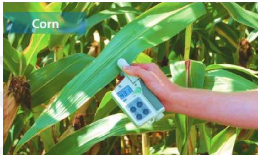
Figure 3.1: Chlorophyll measurement from maize leaf with SPAD-520Plus.
