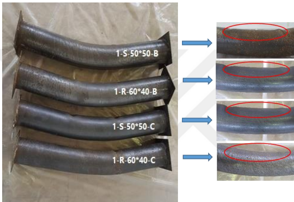
Figure 4.2 Failure patterns of G1.
