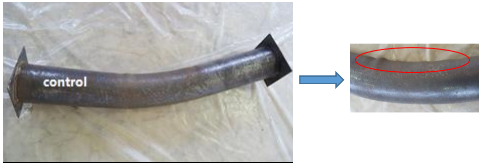
Figure 4.1 Failure patterns of the control.
