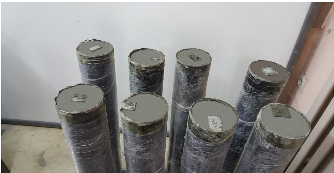
Figure 3.6 The specimens after casting.
