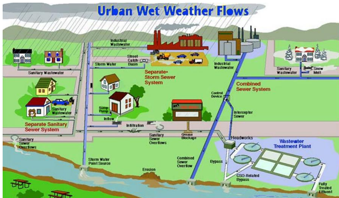
Figure 3.1 : Rainfall-runoff management system.
