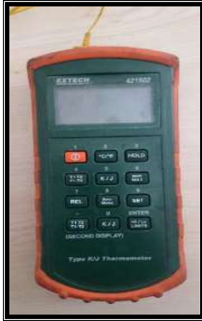
Şekil 5.4 Extech Instruments 421502 Model K/J Tipi Termometre
