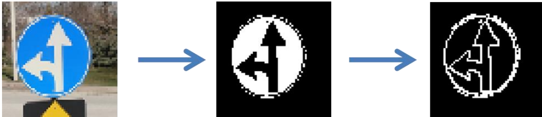
Figure 3.9: Edge extraction for a blue circular traffic sign
