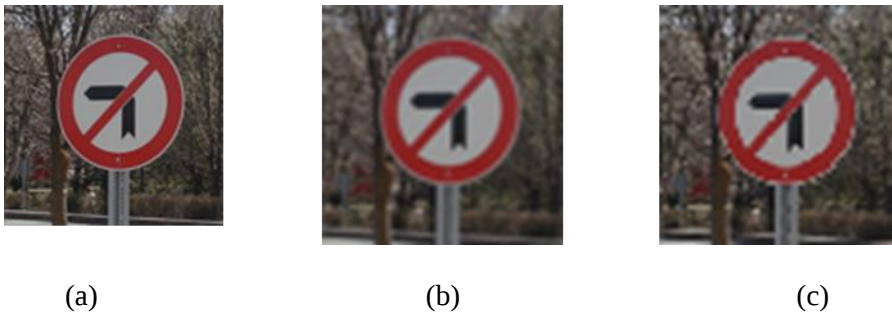
Figure 3.1: Scaling results of a ROI (a) Input image (110x110) (b) Scaling to 60x60 with bicubic interpolation (c) Scaling to 60x60 with the nearest neighbor interpolation
