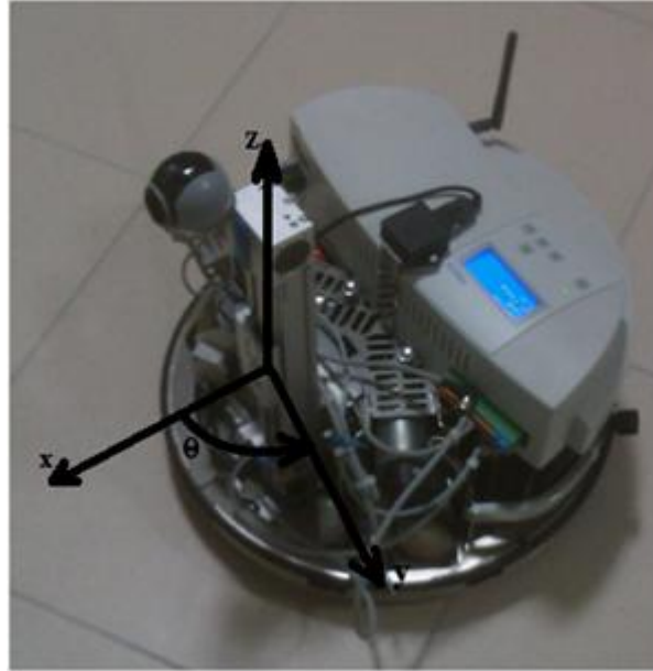
Figure 4.3 Degree of Freedom (DoF) of the Robotino ® .
