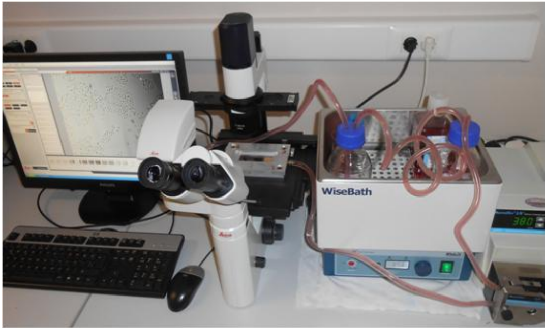
Figure 3.2 Experimental setup showing the HUVECs under flow in branched kit of parallel plate flow chamber connected to peristaltic pump under microscope.
