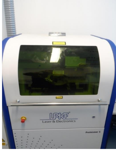
Şekil 3.12. Laser Circuit Structuring LPKF ProtoLaser S
