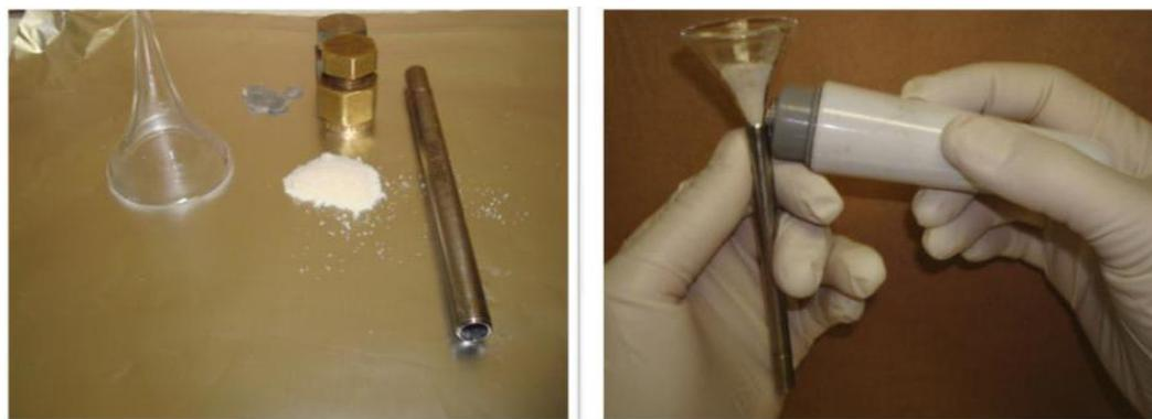
Figure 0.4: Sampling tubes filling process (Civan, 2010)
