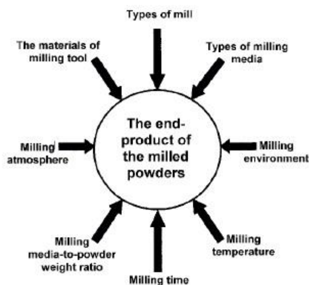
Figure 3.5: Schematic presentation of the main factors that affect the milling process (El-Eskandarany, 2001).
