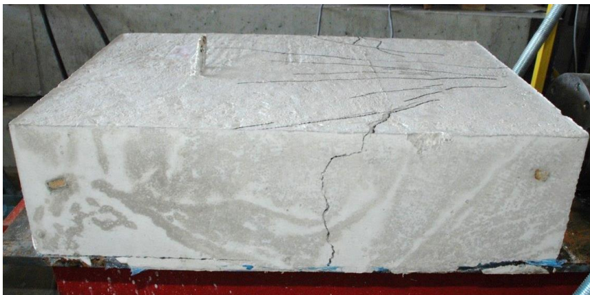
Figure 1.20 Surface Cracking – U140 x 75mm
