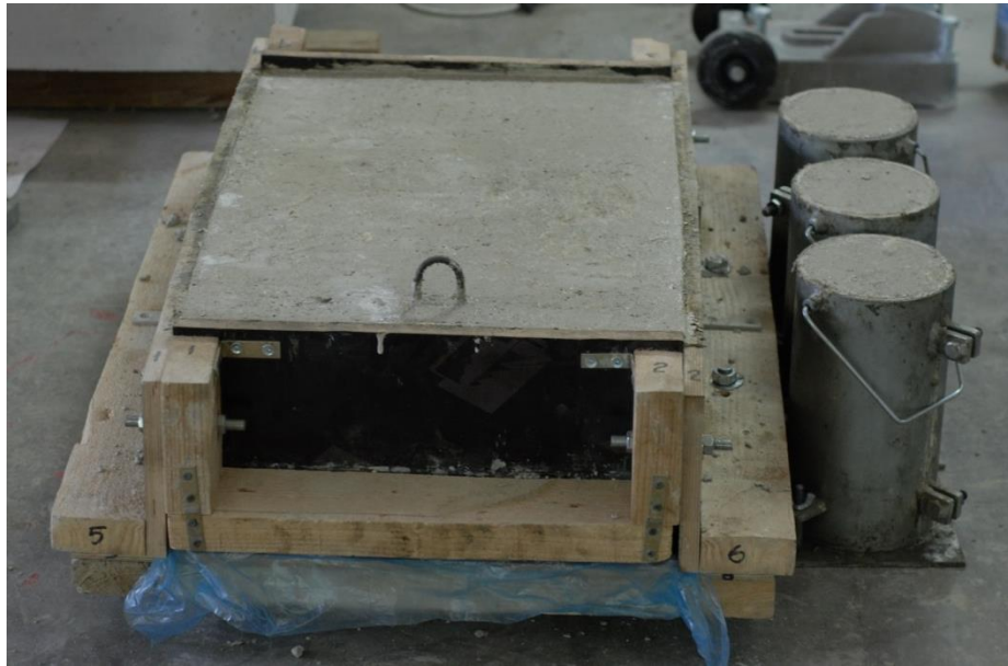
Figure 1.13 Push-Out Specimen and Cylinders
