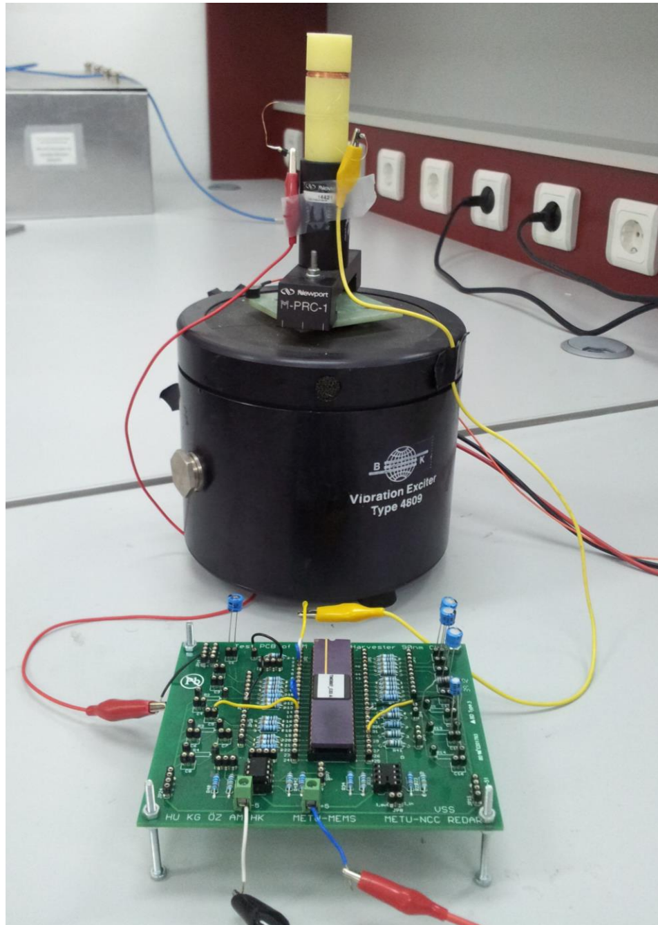
Figure 4.8: The test setup of the TSMC 90 nm chip with the test PCB and the energy harvester.
