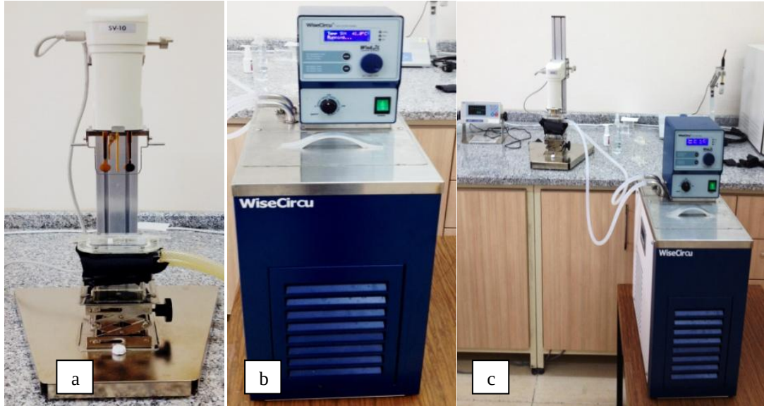
Figure 20. a) The Sine Wave Vibro Viscometer SV-10 (with black insulation on its sample cup), b) the WiseCircu circulating water bath WCR-P8 and c) the viscometer and the water bath.
