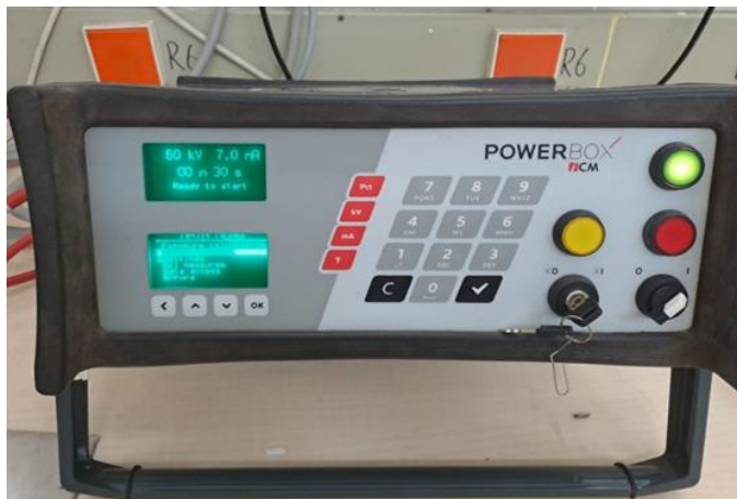
Figure 5.5 : Operating parameters of the radiological imaging device.
