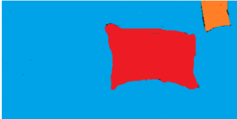
Figure 3.9. C. Cell probabilities (is there a possible detectable object inside this cell): red color for car object, orange color for traffic light object and the blue color for background.
