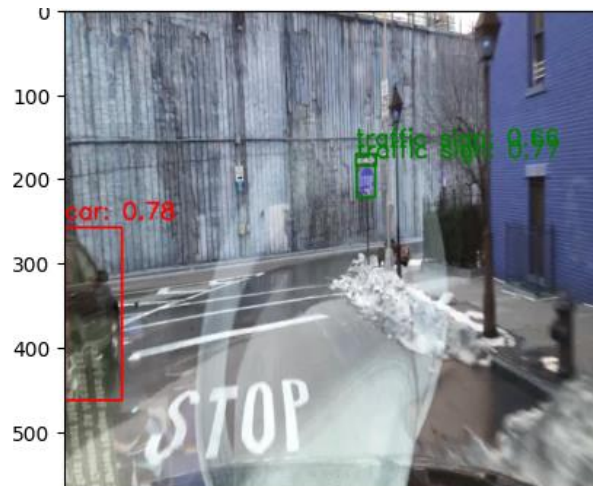
Figure 4.41. A visual detection results of a test sample (example8) (b) Output of detection system (yolo)
