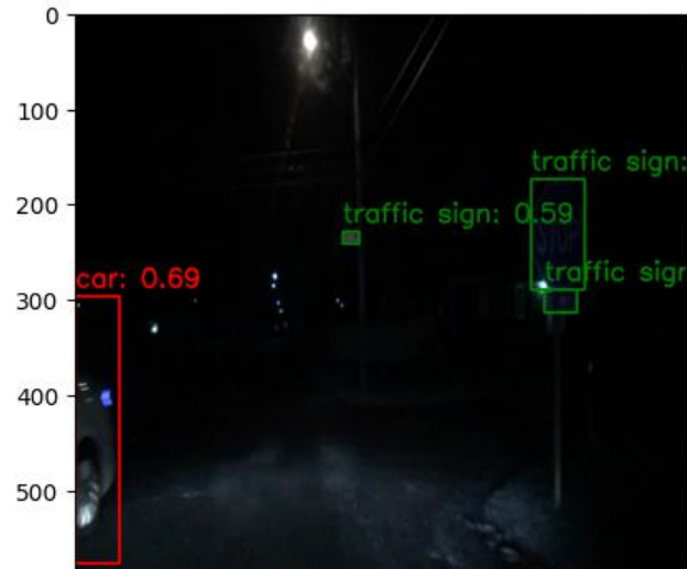
Figure 4.31. A visual detection results of a test sample (example3) Output of detection system (yolo).
