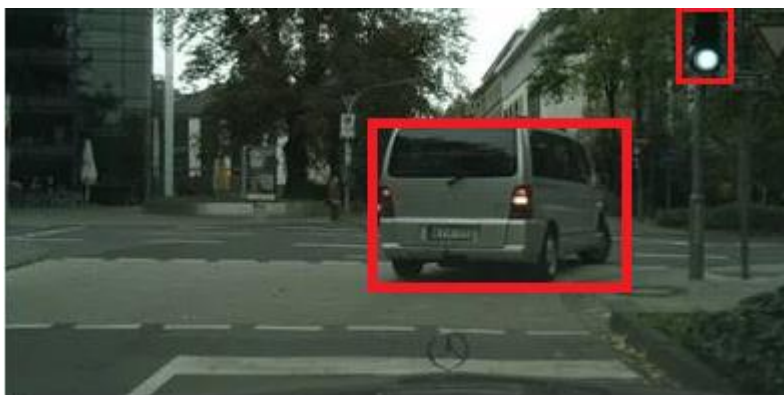
Figure 3.11.E. Detected bounding boxes using a non-maximum suppression operation to find the most appropriate bounding boxes and eliminate outliers
