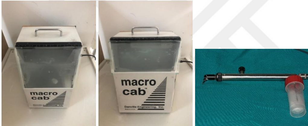
Resim 3.20. Kumlama kabini (Macro Cab, Danville Engineering, ABD), kumlama cihazı (Hager Werken Air-Sonic, Almanya)
