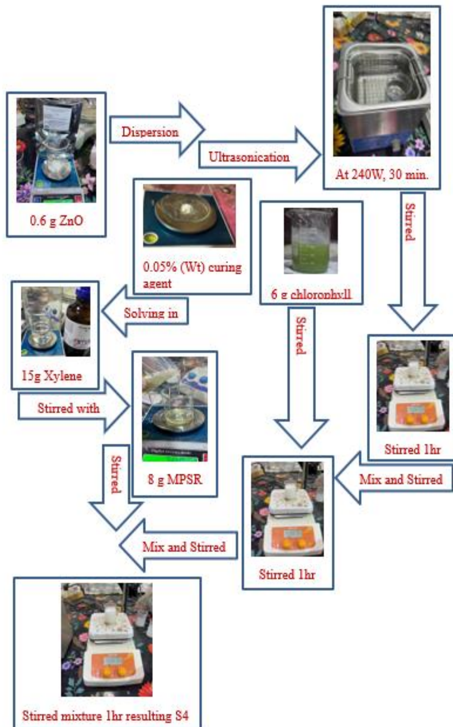
Figure 3.10. Steps preparation S4 (MPSR-chlorophyll-ZnO -SiO 2 coating).
