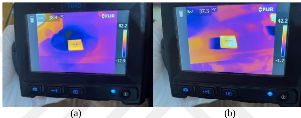
Figure 4.26. Measuring operation temperature surface of mini solar panel for (a) uncoating (b) coating panel.
