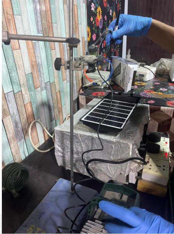
Figure 5.1. Application method for coating on street lamp solar panels.
