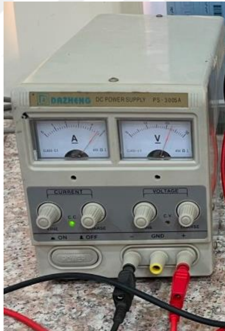
Figure 4.22. Power DC supply.
