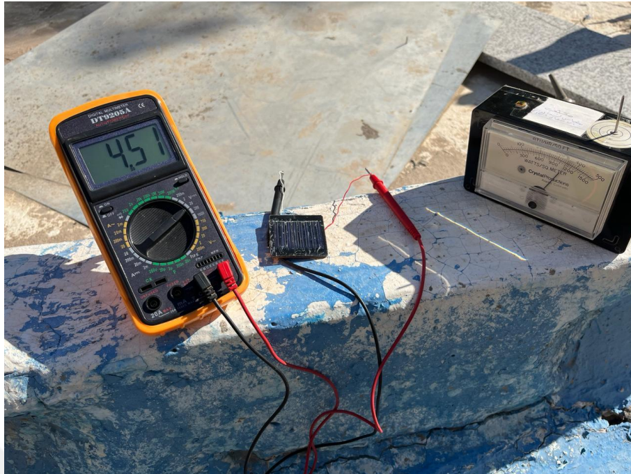
Figure 4.28. DC voltage measurement of uncoating mini solar panel.
