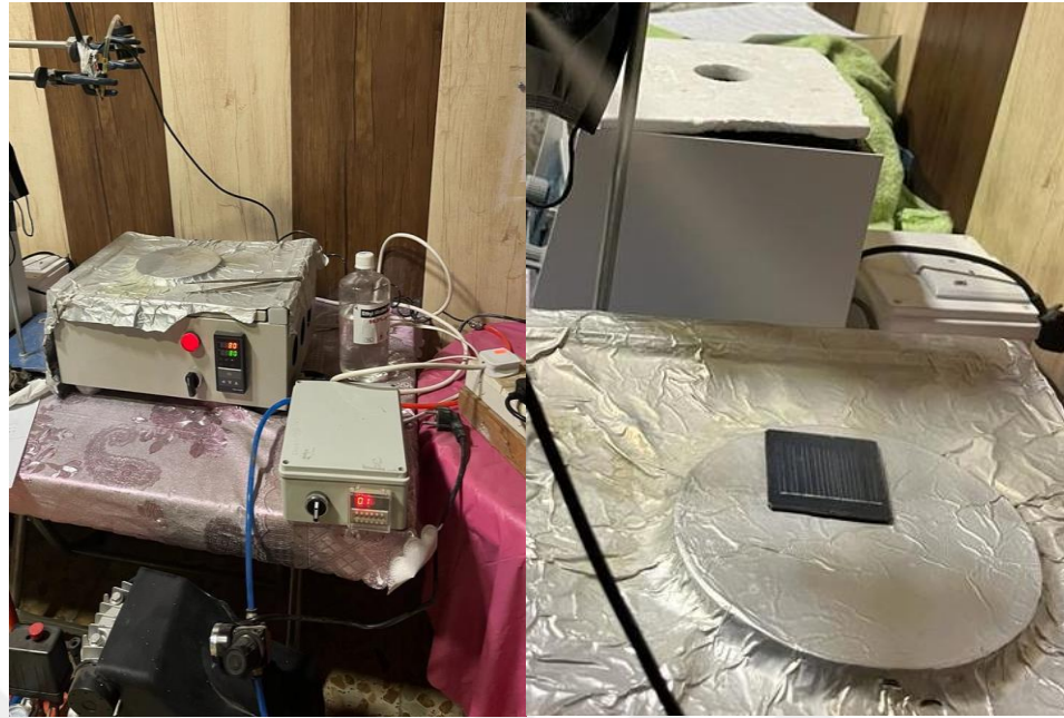
Figure 4.21. Process of coating mini solar panel by spray method.
