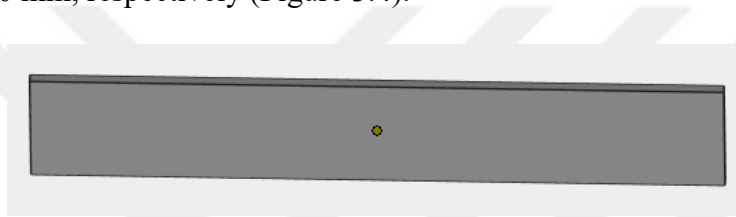
Figure 3.4 : Sample design that is used to determine roughness measurement method. Thickness is 1 mm, width is 12 mm and length is 70 mm. 6 of this sample design are produced within the same region (right bottom corner) of the build plate.
