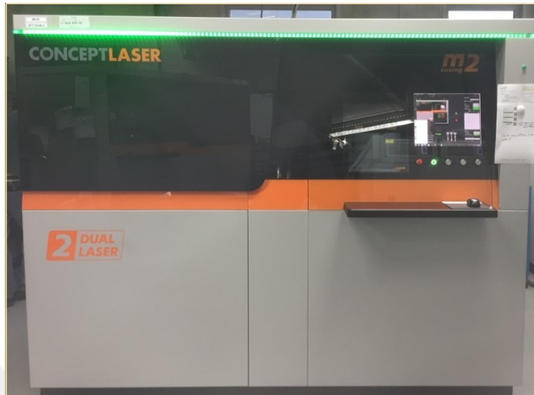
Figure 3.1 : Selective laser melting machine (M2 cusing GE Concept Laser).
