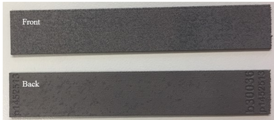
Figure 4.1 : Front side of the sample displaying rougher appearance than the back side.
