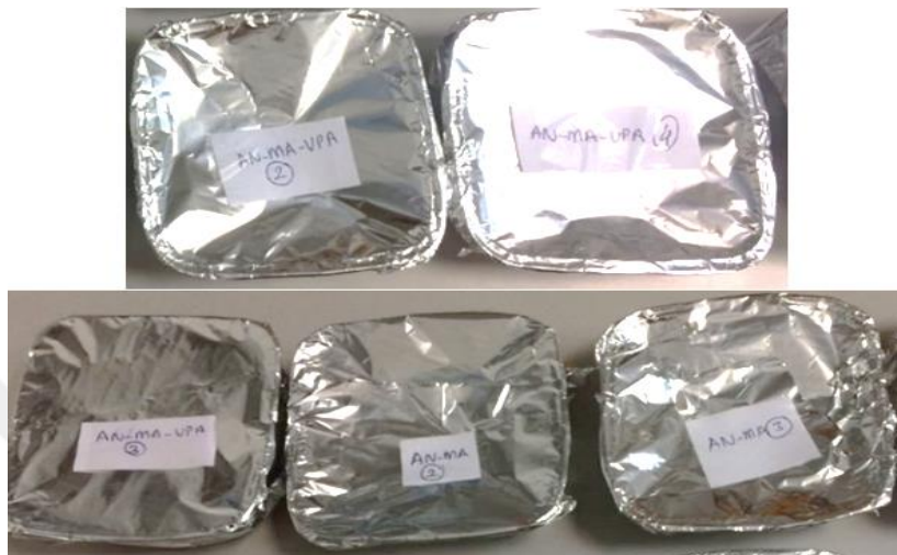
Figure 3.6 : Water absorbance test cups
