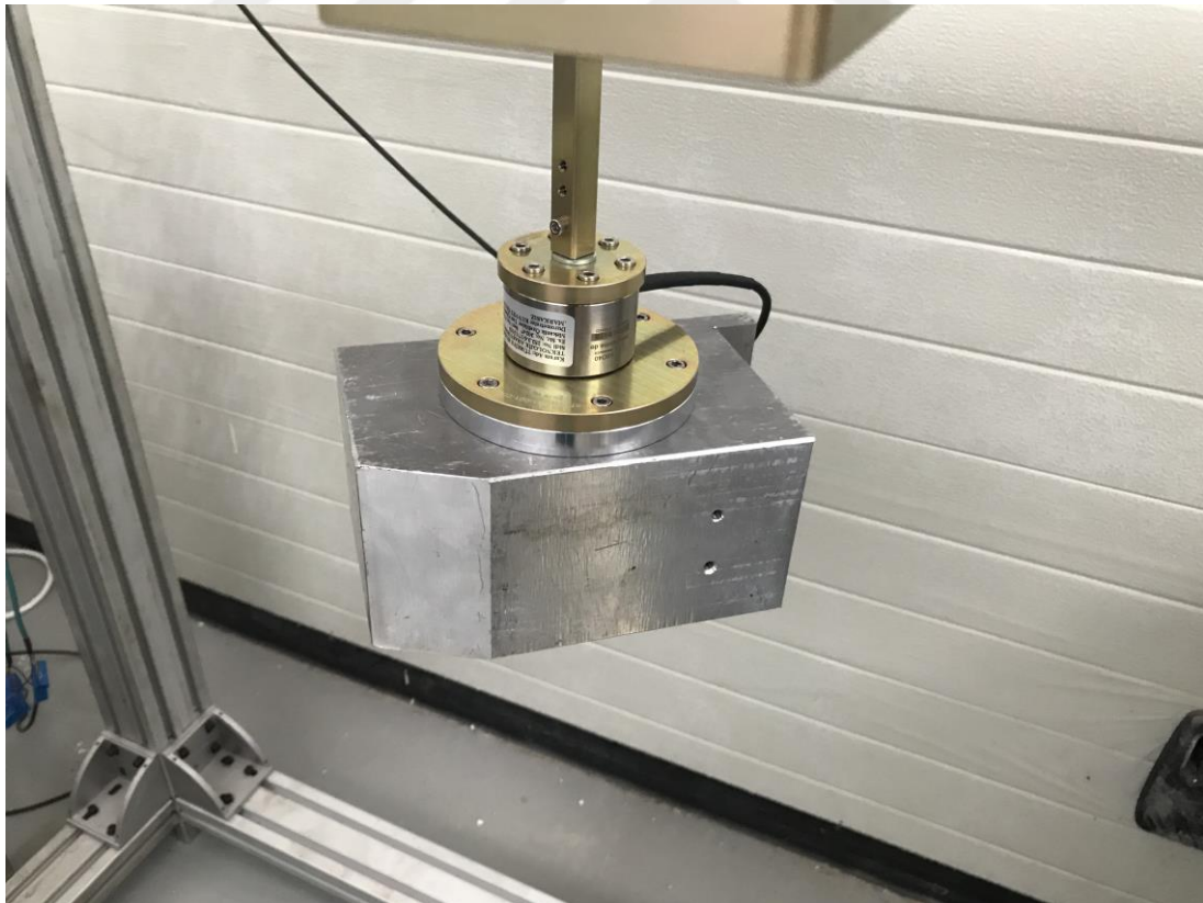
Figure 38. Shown aluminum block is used to measure mass properties.
