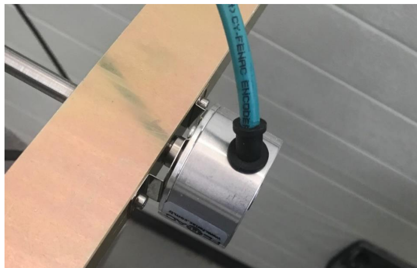
Figure 32. Encoder and connection to the frame is shown.
