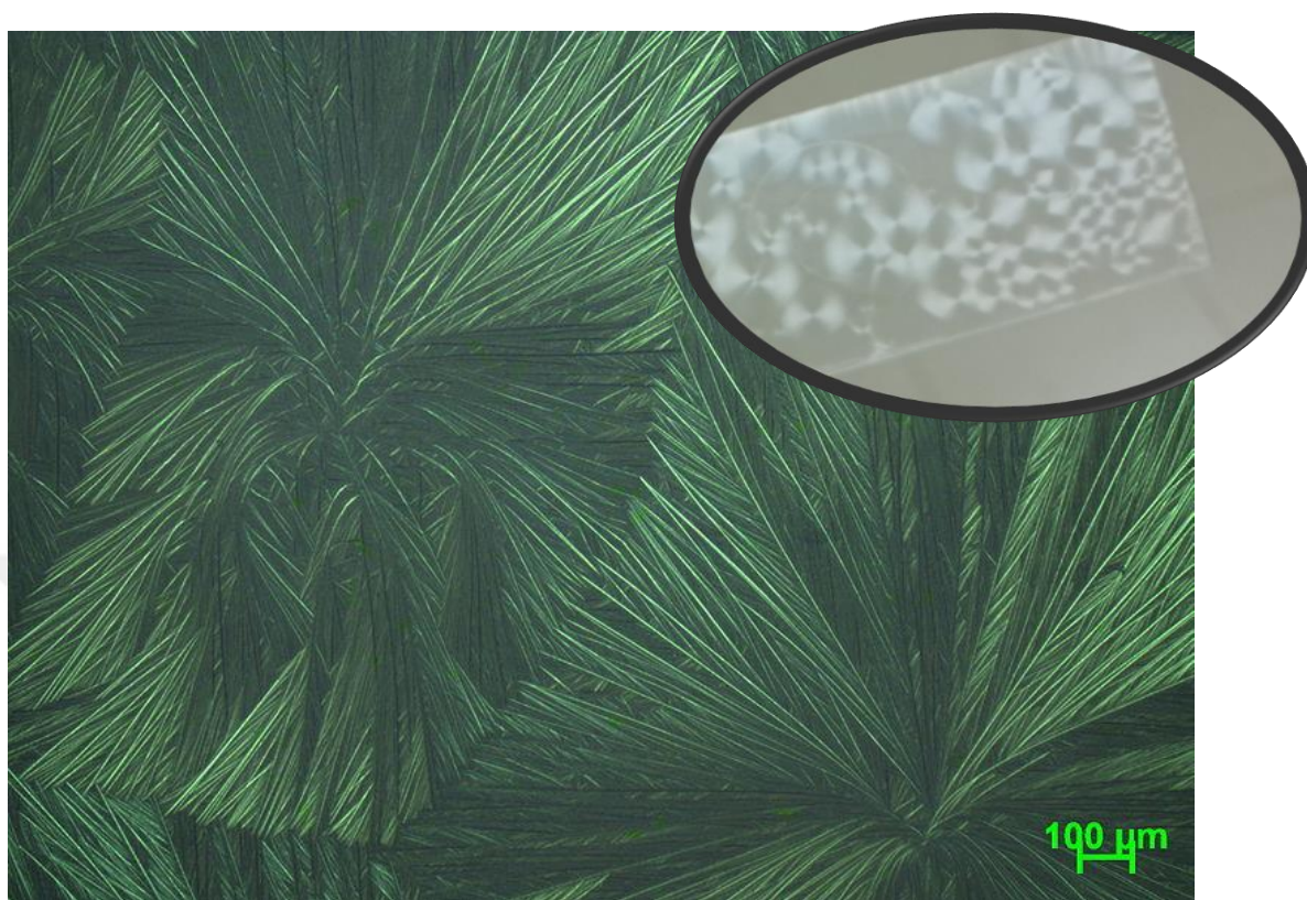
Figure 3.1.3.1. The POM image [76] and the photograph of the drop casted films from 6:2 solution. 9
