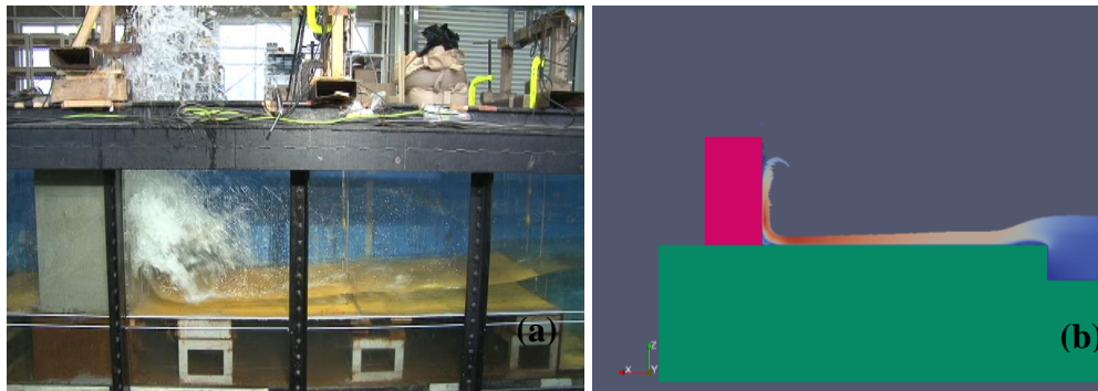
Figure 4.22. Snapshots from (a) the video of the experiment (Arikawa, 2015) and (b) simulation video of the k-\omega -SST turbulence model for Case 3
