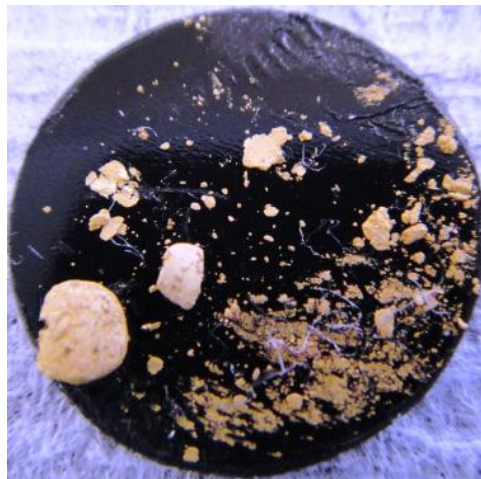
Picture 8 SEM test sample; gold particles on carbon sticky
