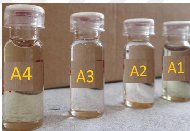
Picture 2 One set of X-ray exposed tubes after a while from exposure (A4 is in intense colour due to gold nanoparticles)
