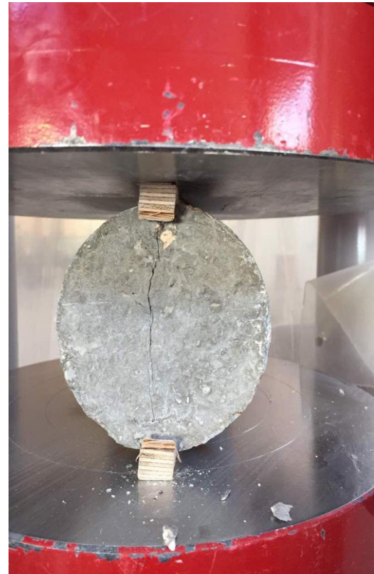
b. Sample after crush
