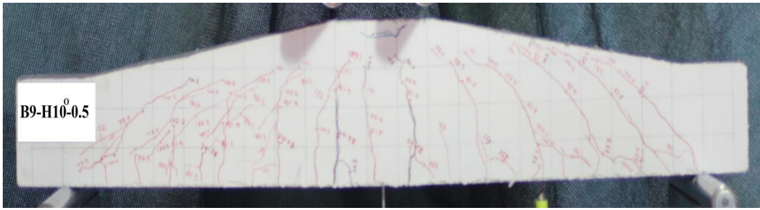
Figure 4.19 Flexural Failure Mode
