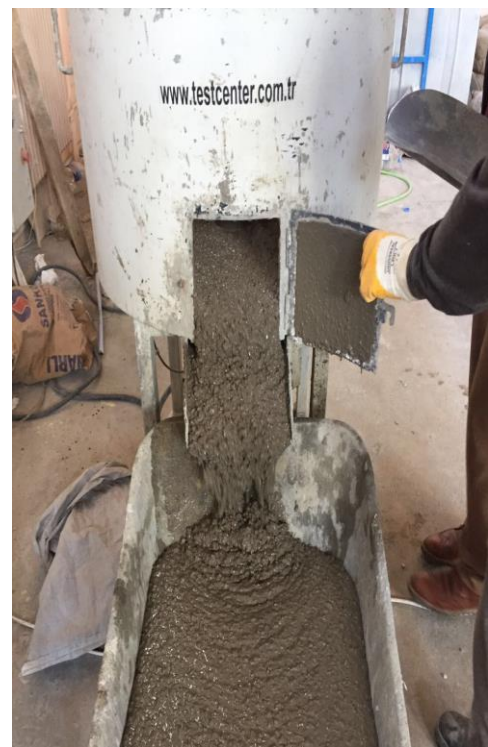
b. Concrete dump
