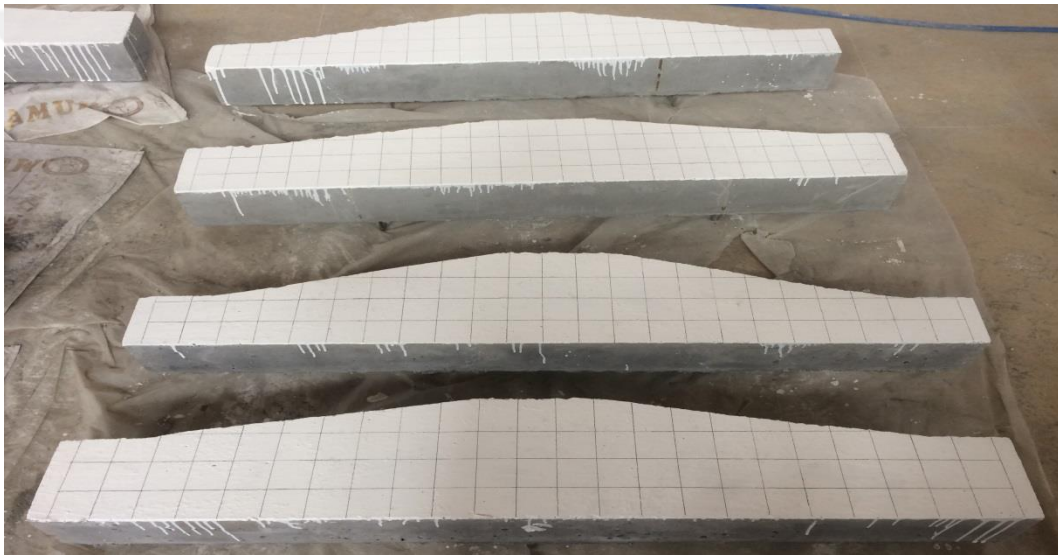
Figure 3.16 Preparing beams for test
