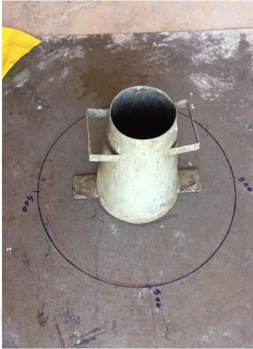
a. Slump flow test and T50 apparatus
