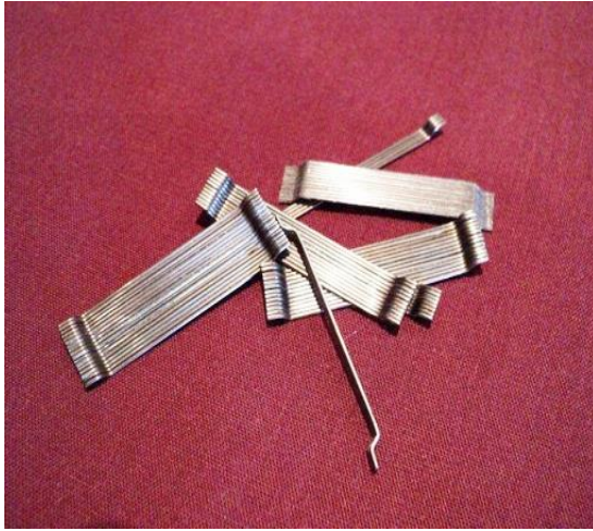
a. Shape of steel fiber
