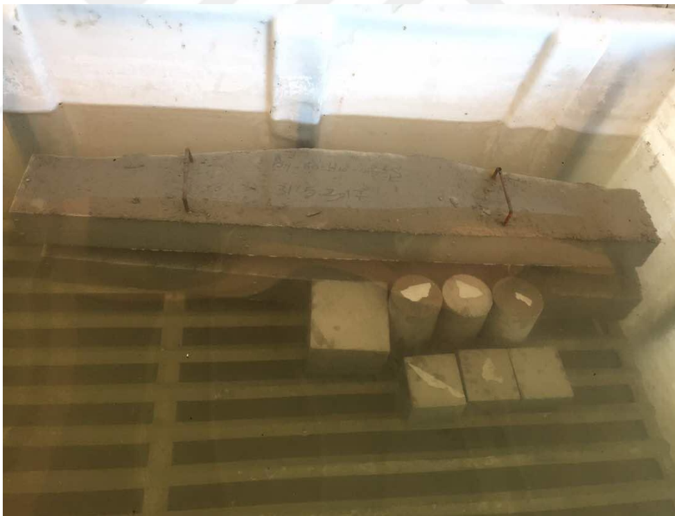
Figure 3.15 Curing beams and samples 28 day
